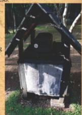
Charcoal is ideal because it is porous and readily available. The black color of the charcoal absorbs heat from the sun that helps to evaporate the water that carries with it the heat, creating the cooling effect.
